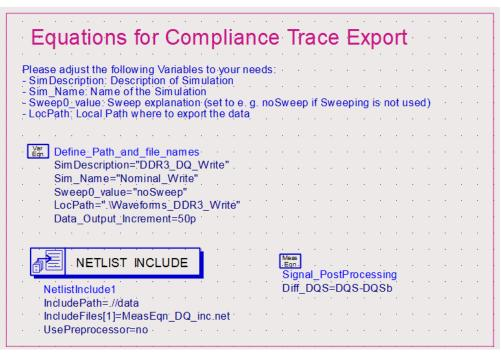
The IncludeFiles[1] refers an ADS netlist , i.e., MeasEqn\_DQ\_inc.net, which writes a set of waveforms to *.hdf5* files. For example, the following AEL Expression (aele) statement in *MeasEqn\_DQ.net* file, writes a schematic node name *DQ0* (1<sup>st</sup> argument) into a file named *DQ0.h5* (2<sup>nd</sup> argument). This is located in a folder specified by LocPath (3<sup>rd</sup> argument):
