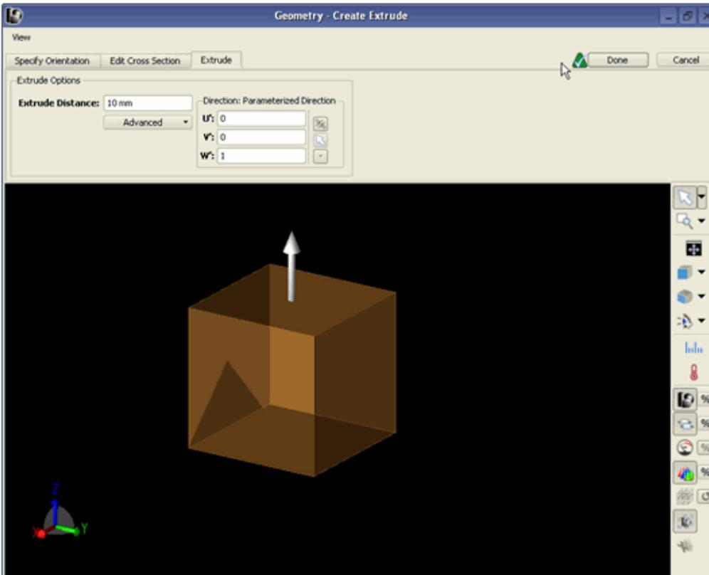
9. Enter a value in the in the **Extrude Distance** text box. You can also move the arrow
