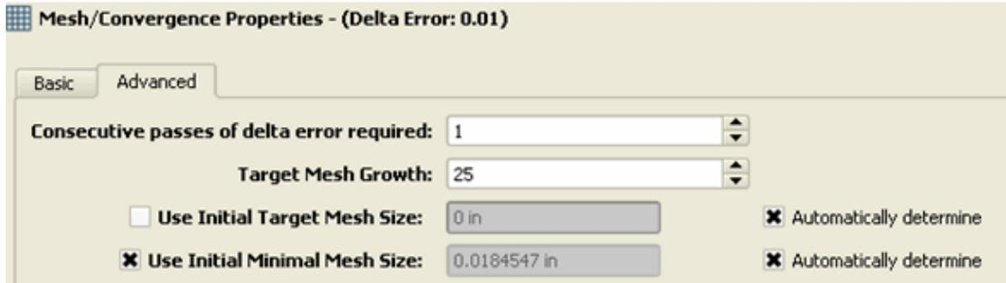
The figures below illustrate the effect on a simple example when the setting minimum size is not set.
