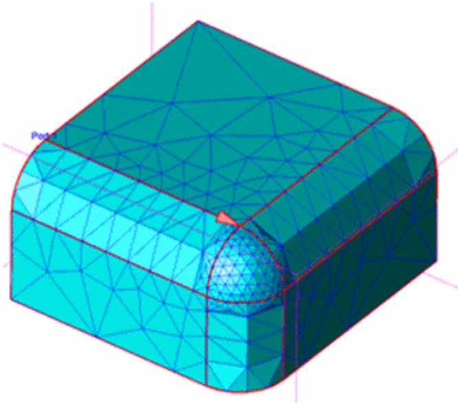
The figures below illustrate the effect on a simple example when the setting minimum size is set to 3 mm.
