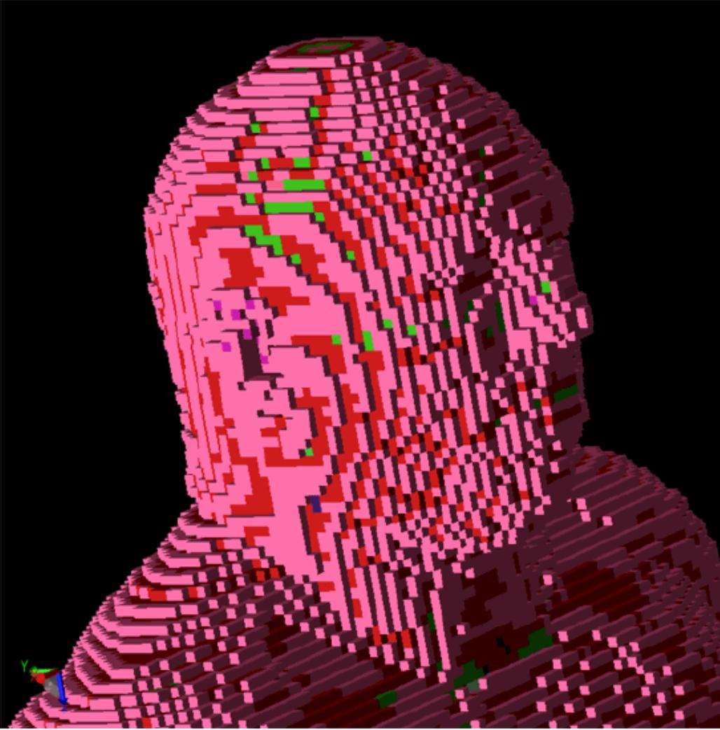
The following illustration shows the *Project Tree* after the the \*.mmf file seen above was imported. Note that an object has been added to the *Parts* branch that contains the voxel object and a list of all the materials contained in the object have been added to the *Definitions: Materials* branch.
