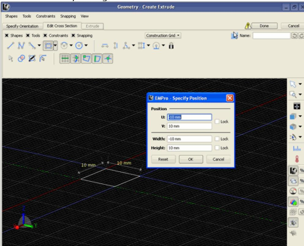
6. Extrude it to create a 3D object. Select the required coordinates or press **Tab** to open the **Specify Position** dialog box.
