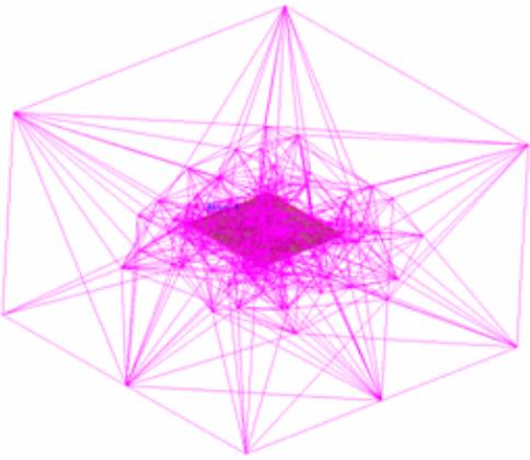
When the same volume is meshed using the **Initial Target Mesh Size**, the mesh looks like:
