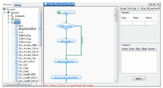
The extraction flow has hierarchical structure. You can create several task groups in one flow and make the flow clearer and more readable. The tasks need to be written by script. For more details, refer to the MBP Script Application Manual.
