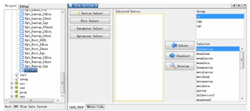
To deselect a device selector, firstly click on the selector in the Selected Device list, and then click on Deselect Button. We could click on Preview button to view the selection in geometry plot. The selected devices will show by filled points.
