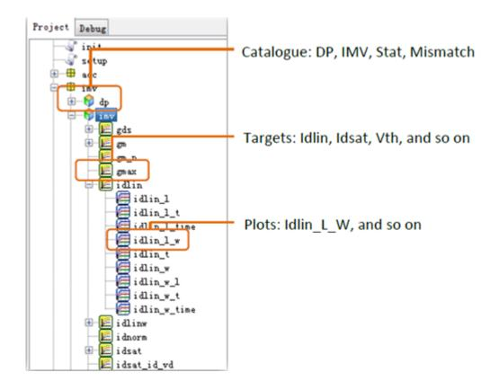
The hierarchical structure of IMV is shown above. For each catalog, there are different targets defined by users (MBP provides default settings and the configurations are fully open to users.)
