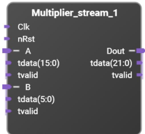
Multiplier (DSP core) with streaming interface.
