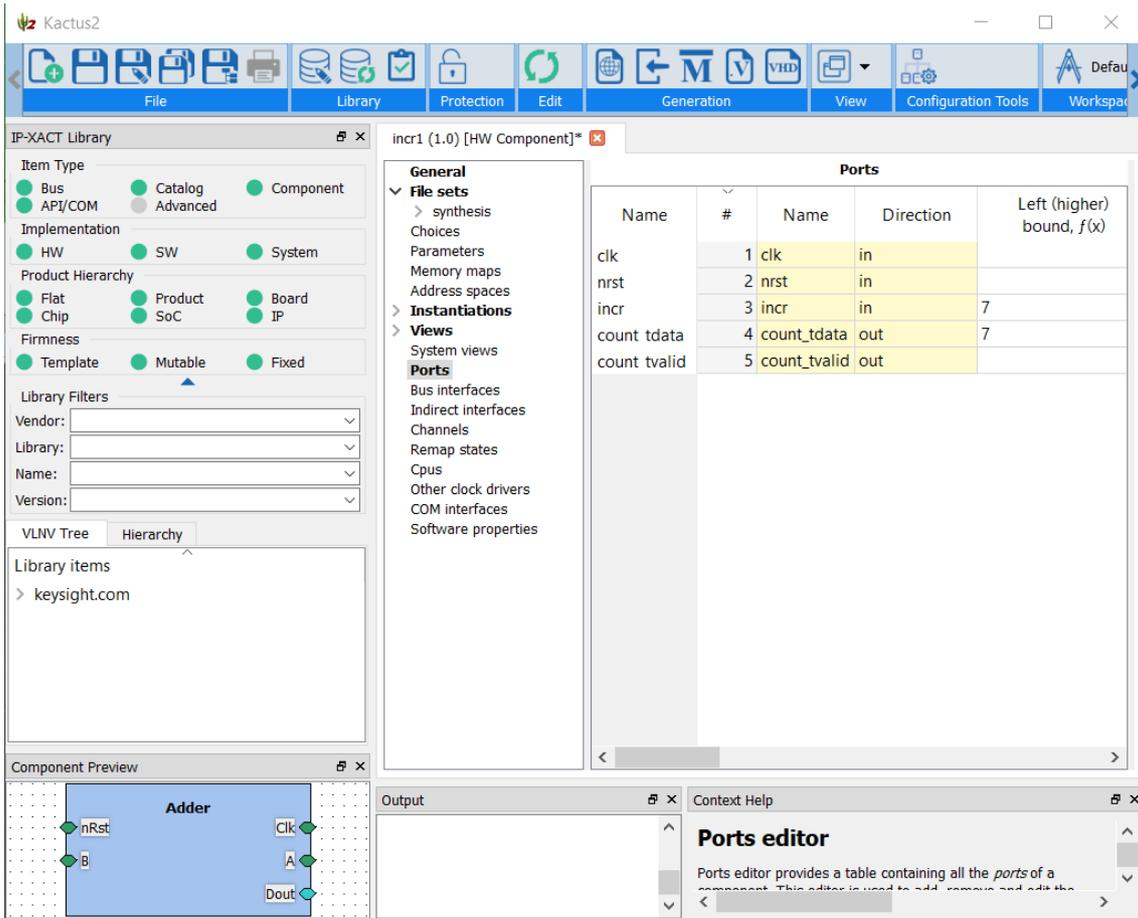
To assign a single port to an interface, select the port in the yellow box under the **Name** column, right-click and select **New bus interface/Use existing bus definition**.
