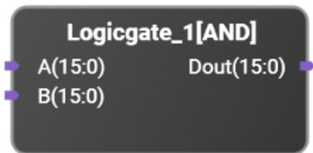
Output is the logical operation between inputs A and B.
