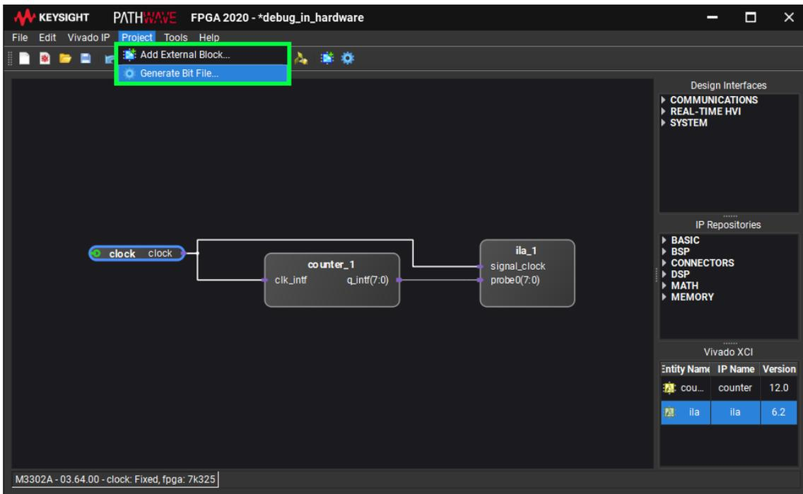
Next click on Generate Bit File and then click the Run button to run synthesis for the Pathwave FPGA project and to generate the bit file.
