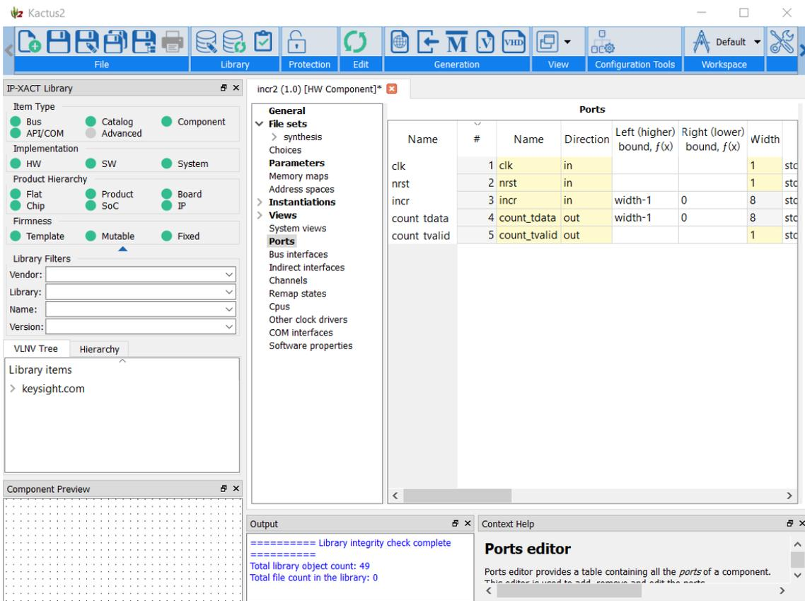
To assign a single port to an interface, select the port in the yellow box under the **Name** column, right-click and select **New bus interface/Use existing bus definition**.
