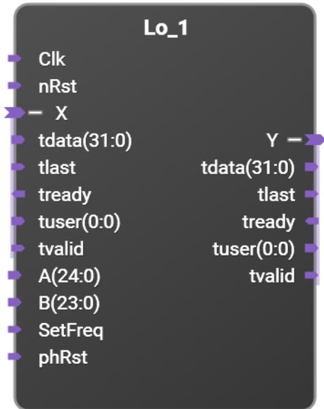
This block supports supersampled data. In this description let  $S$  be the supersample factor. For non-supersampled data, set  $S$  to 1. The bit width of each data sample can be changed via the "Tdata size" parameter. Note that this parameter denotes the width of each individual sample, not the supersampled data width. The width of a real tdata port will be  $S$  times the Tdata size parameter while the width of complex tdata port will be  $2S$  times the Tdata size parameter.
