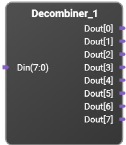
Converts a single N-bit input vector into N single-bit output signals.
