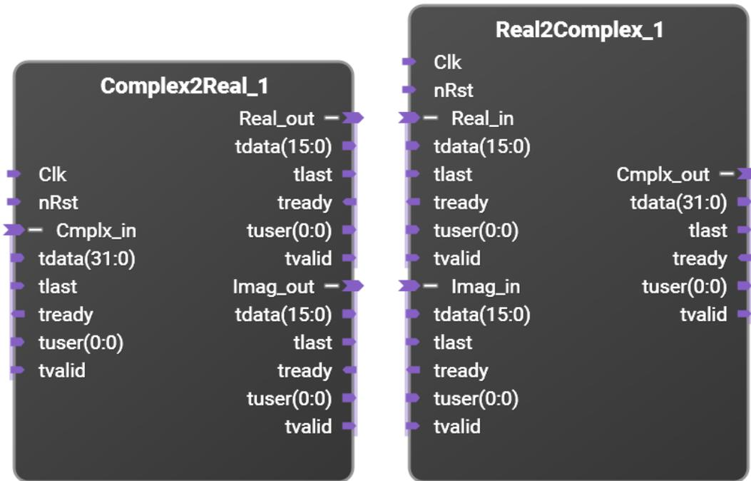
Converts between one complex stream of data using interleaved real and imaginary parts and two separate streams, one for real and one for imaginary parts. These can be used to split off the real and imaginary streams into different destinations or to combine two real streams into one complex stream.
