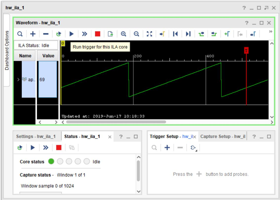
Without any trigger setup, the trigger position is random. However, the Xilinx ILA debug core supports advanced trigger setups. As an example, adding a trigger can stabilize the trigger position within the repetitious waveform.
