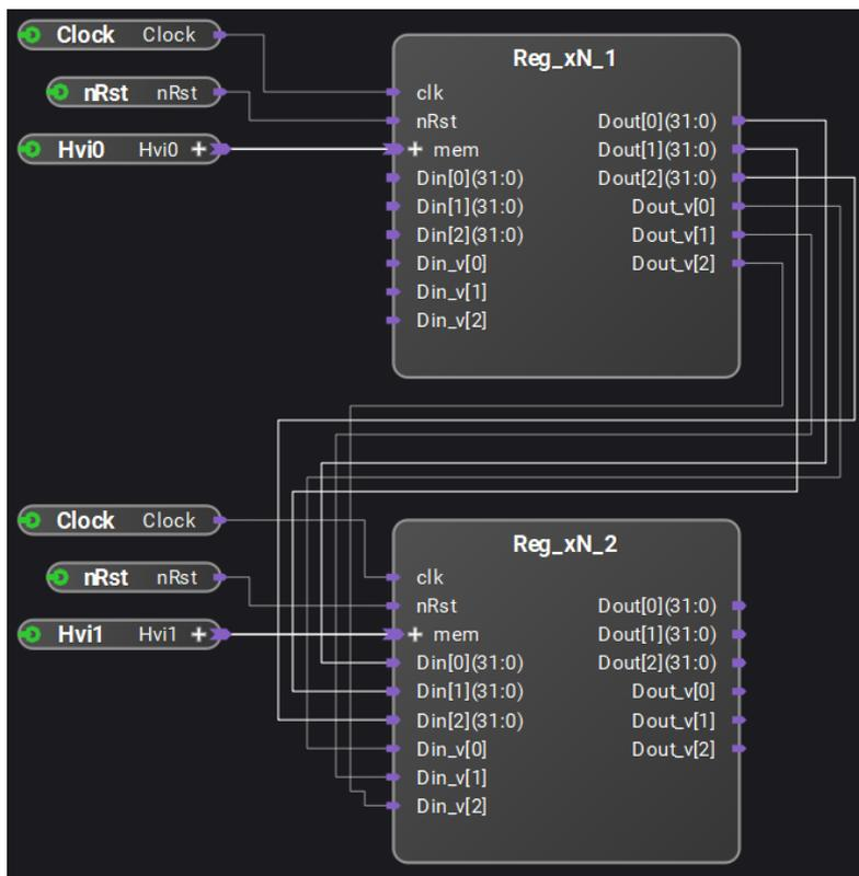
The PathWave FPGA project instantiates two register blocks each with three registers. The first register block (Reg\_xN\_1) connects to an HVI port called Hvi0. The second register block (Reg\_xN\_2) connects to an HVI port called Hvi1. The register output from Reg\_xN\_1 is connected to the register input of Reg\_xN\_2. This allows the HVI code to write values to Hvi0 and read back the values at Hvi1.
