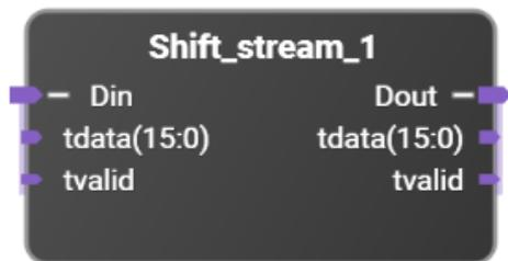
Signal shifter with configurable input size, direction and number of shifts using streaming interfaces.
