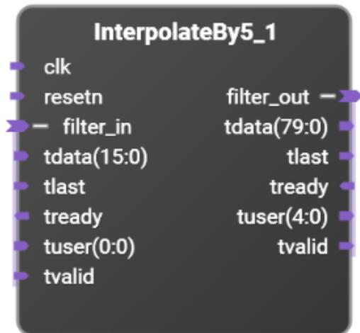
Interpolate an input stream by a factor of 5. Interpolation is achieved using an oversampled, FIR filter.
