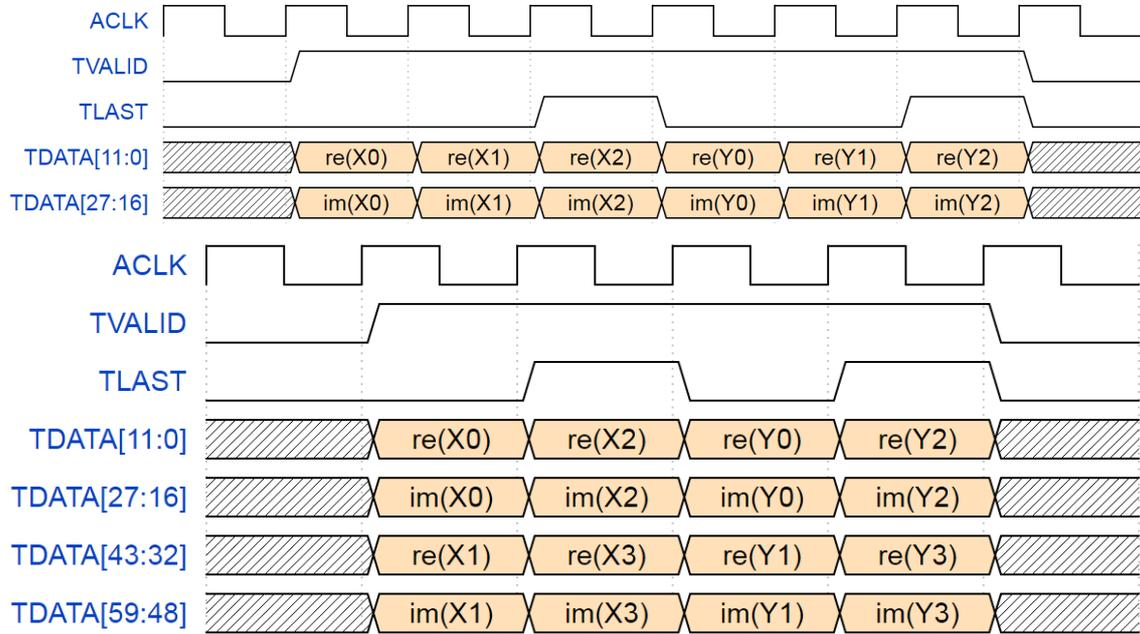
Above are examples of parallel complex data (one sample per clock and two samples per clock). Below is an example of serial complex data.
