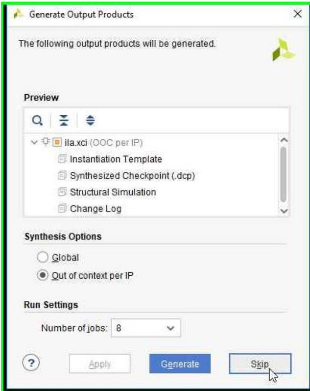
Click the Skip button to skip generation of the customized ILA IP core output products for now. The XCI file is all that is needed to import the component into PathWave FPGA and the output products for any customized IP cores are automatically generated later when building the PathWave FPGA Sandbox design. Then close/exit the Vivado IP Manager to return to the PathWave FPGA window.
