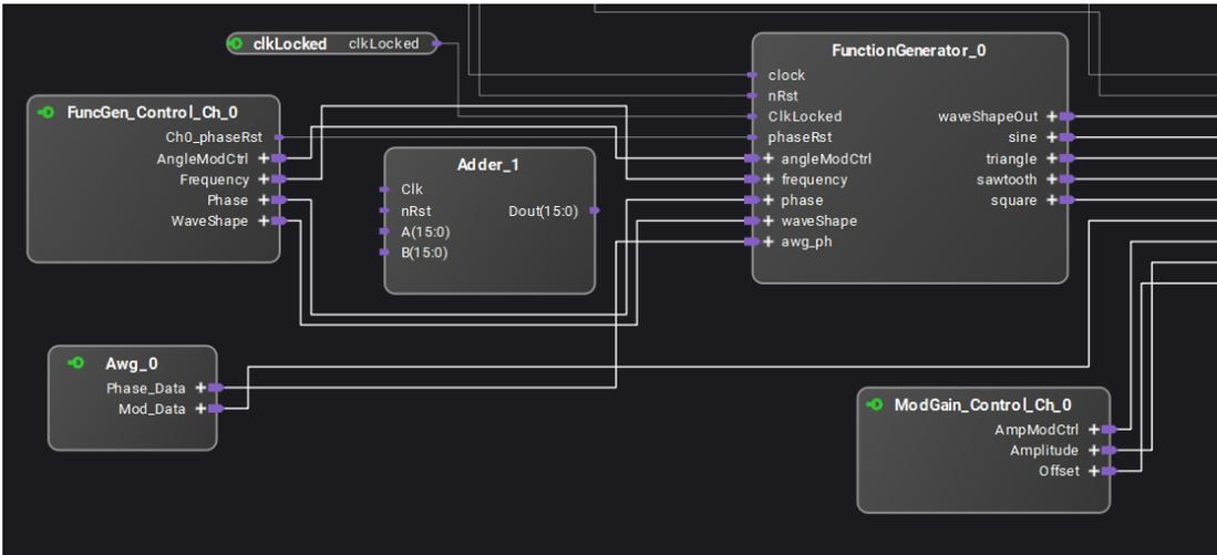
Delete the block that was just added and notice that the connecting line stays unchanged. Right-click the line and select **Redraw**. The line will be straight again.
