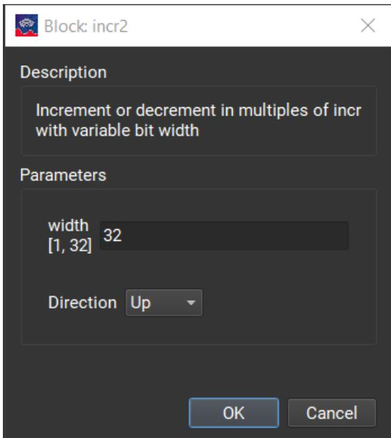
In this example, the user changed the *width* parameter from the default value of 8 to the value 32. This causes the I/O ports to have a range of (31:0) rather than (7:0).
