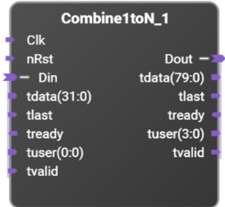
Combines N AXI-streaming samples into one AXI-streaming sample that is N times wider. The input is not supersampled while the output is supersampled by N.
