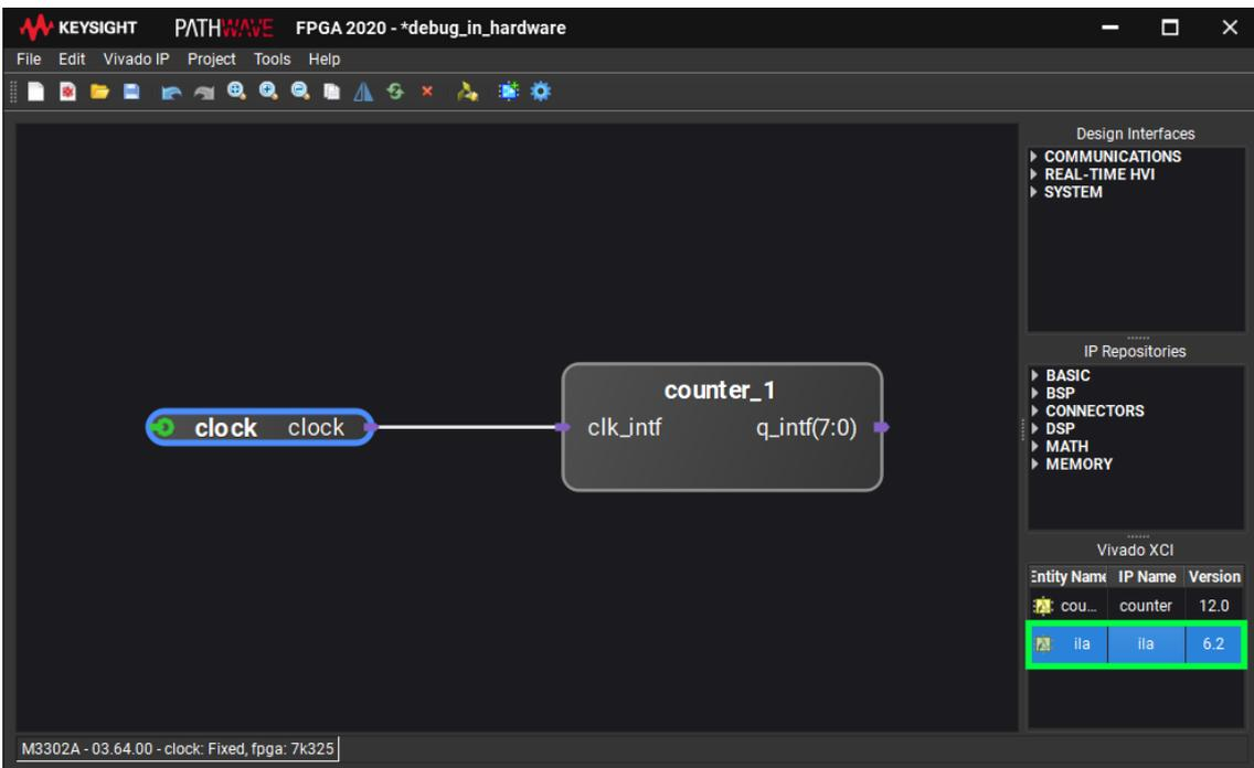
In the Vivado XCI panel, double click on the customized ILA IP core to instantiate the ILA in the Sandbox design. Then make the necessary signal connections of the ILA core to the clock and counter output, as shown below
