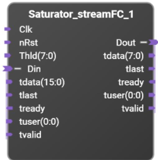
Data saturator with streaming interface with full flow control support.
