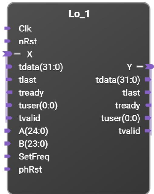
Parameterized Local Oscillator. It handles supersampled or non-supersampled data, and either the input and/or the output can be real or complex.
