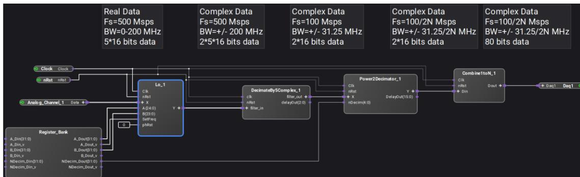
In this example, the input ADCs of the M3302 are running at 500 Msp/s. The FPGA only runs at 100 MHz, so the input (Analog\_Channel\_1) presents 5 ADC samples every FPGA clock. This is called supersampling by 5. The five 16-bit input samples are combined into one 80 bit wide AXI-streaming bus.
