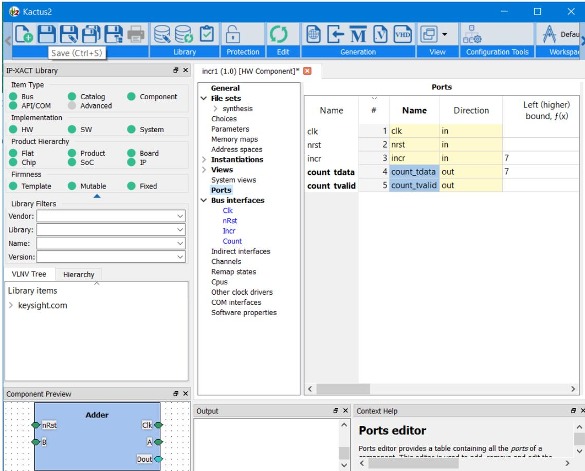
The description of this block's interfaces is now complete and PathWave FPGA can now use this interface information to allow easier connections to other blocks.
