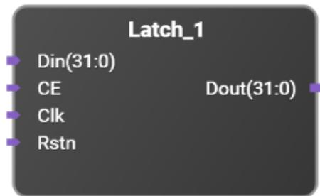
32 bit latch with write enable.
