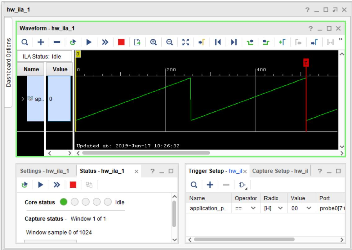
Multiple acquisitions now produce exactly the same acquisition data, with the trigger position stable on counter value equals zero condition.
