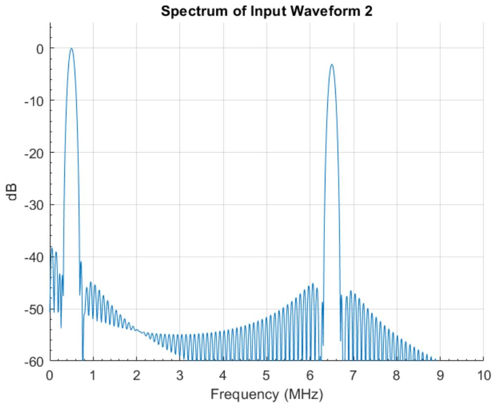
Both of these channels are low pass filtered and then decimated by 8. The 0.5 MHz component of both signals is well within the passband of the decimator and passes through unchanged. The first signal has a tone component at 4.5 MHz. This falls in the transition band
