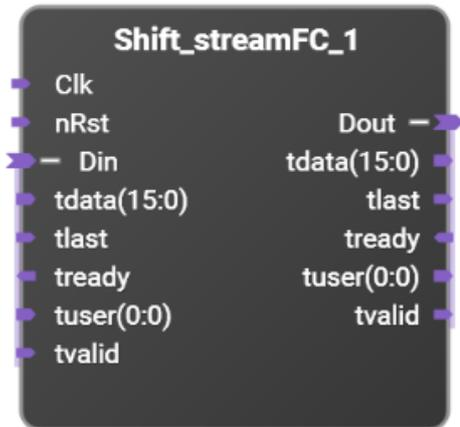
Signal shifter with configurable input size, direction and number of shifts using streaming interfaces with full flow control.
