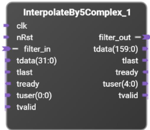
Interpolate a complex input stream by a factor of 5. Interpolation is achieved using an oversampled, FIR filter.
