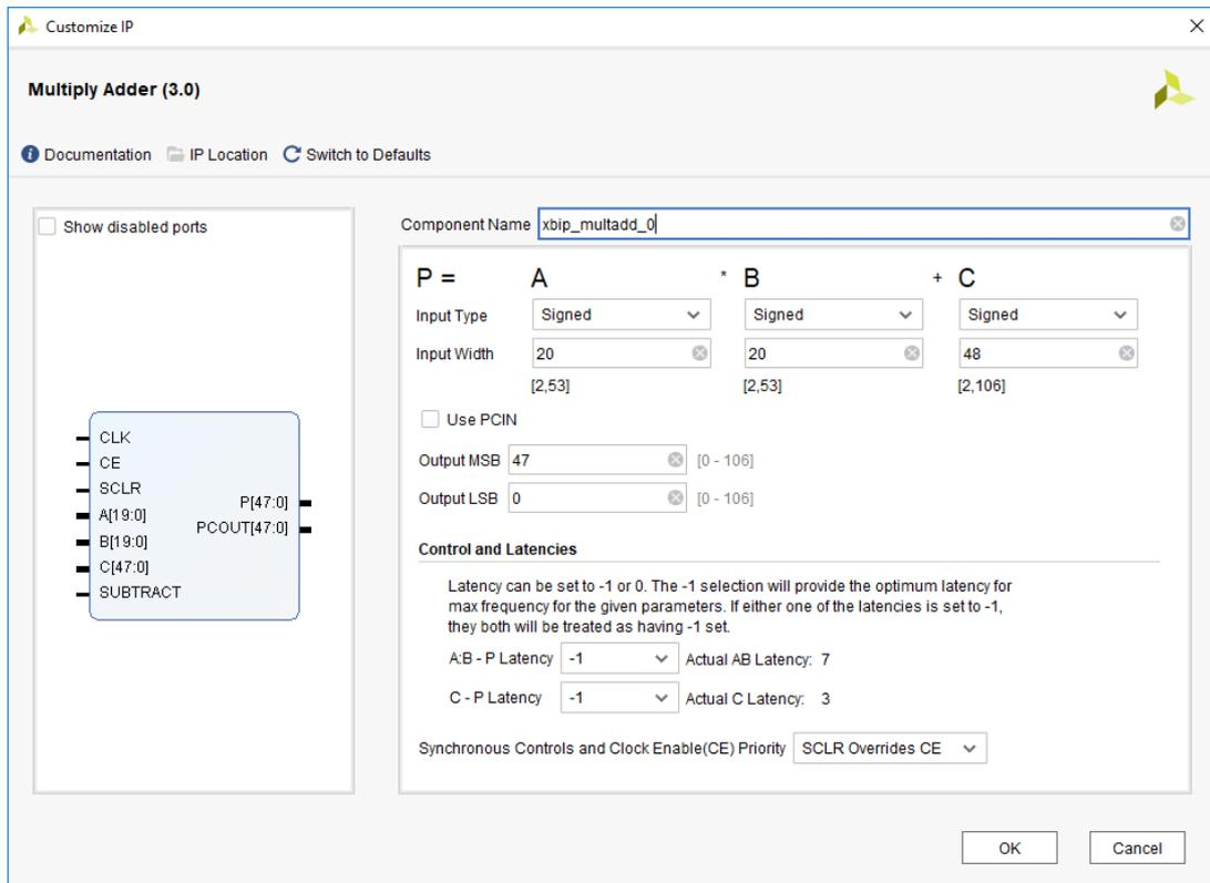
4. Click the Skip button. PathWave FPGA always regenerates Vivado IP during bitfile generation, so the output products created by clicking Generate are not needed.
