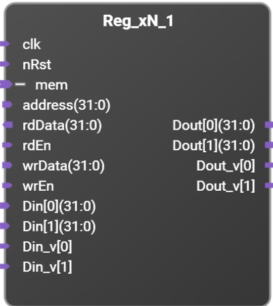
Captures N, 32 bit data inputs and drives to outputs. The internal data register may be updated through a write access on the 'mem' port indexed by the address value. The internal data register may also be updated to the Din value by asserting the corresponding Din\_v signal[n]. When both updates are attempted at the same time, the mem write value will take precedence. The values of the internal data registers are driven out the Dout[n] ports.
