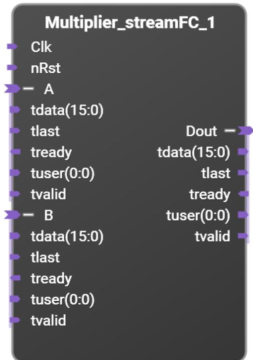
Multiplier (DSP core) with streaming interface and full flow control support.
