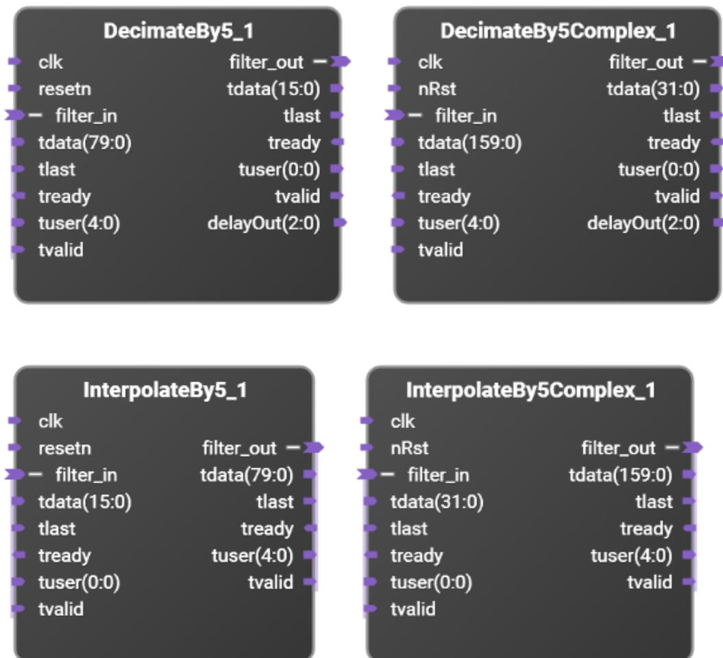
The DecimateBy5 block first low pass filters the input to protect against aliasing and then decimates by 5 (discarding 4 of every 5 output samples). The InterpolateBy5 block first interpolates by 5 by inserting 4 zero samples between each input sample and then low pass filtering to protect against aliasing. Both IP blocks use the same filter which has the frequency response:
