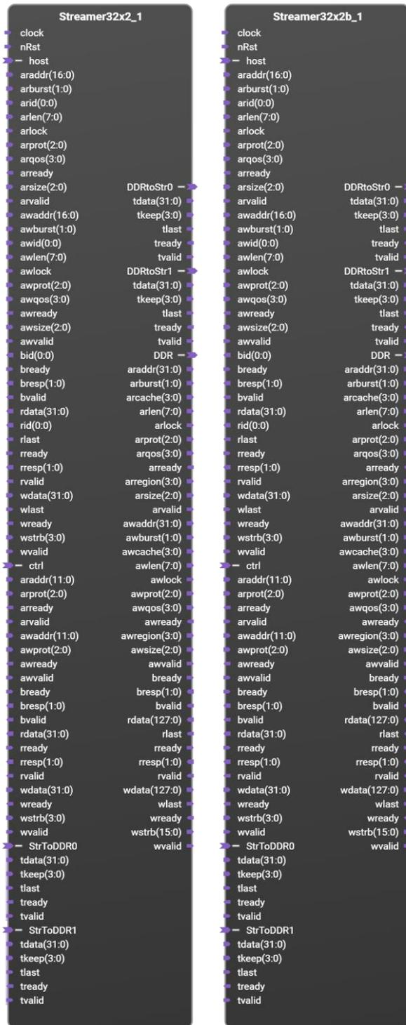
NOTE: The Streamer32x2 IP block uses the Vivado 2017.3 AXI DMA IP block. This IP block has a 23 bit transfer length register. This means the largest DMA transfer size allowed is 8 Mbyte. If a larger transfer size is needed, use the Streamer32x2b IP block. The Streamer32x2b IP block uses the Vivado 2018.1 AXI DMA IP block that has a 26 bit transfer length register. This allows DMA transfers up to 64 Mbyte.
