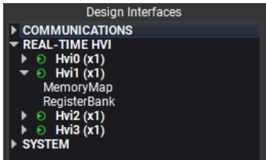
When double-clicking on the *MemoryMap* option, the new interface instance block dialog will appear. In the dialog, the **Entity Selection** section provides a list of available conversions for this interface. The first item in the list is always the type of the design interface. If there is only one available option (i.e. only the design's interface type), then this one is automatically picked and the Entity Selection section is not shown.
