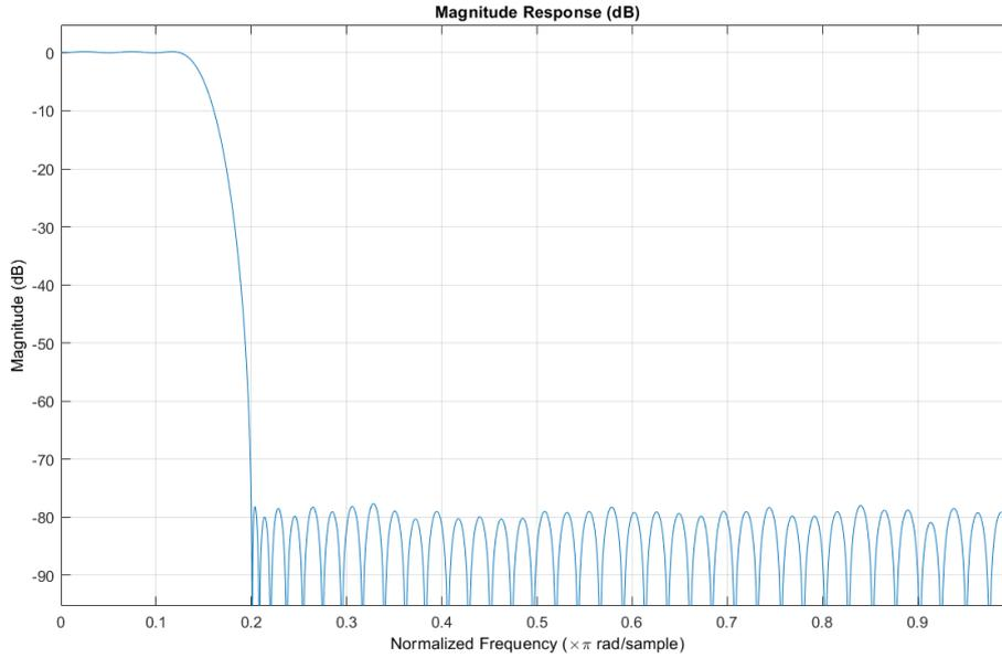
Note that the x-axis is in terms of the normalized frequency where 1 means  $f_s/2$ . The passband extends up to 0.125 with the stopband starting at 0.2. For example, the M3102 digitizer has a sample rate of 500 Ms/s. Thus  $f_s/2$  is 250 MHz and the passband is +/- 31.25 MHz with the stopband above 50 MHz. Note that these numbers are only for a sample rate of 500 Ms/s. For other sample rates, the passband and stopband frequencies would scale accordingly.
