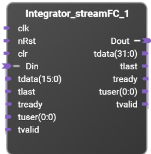
Data integrator with streaming interface with full flow control support.
