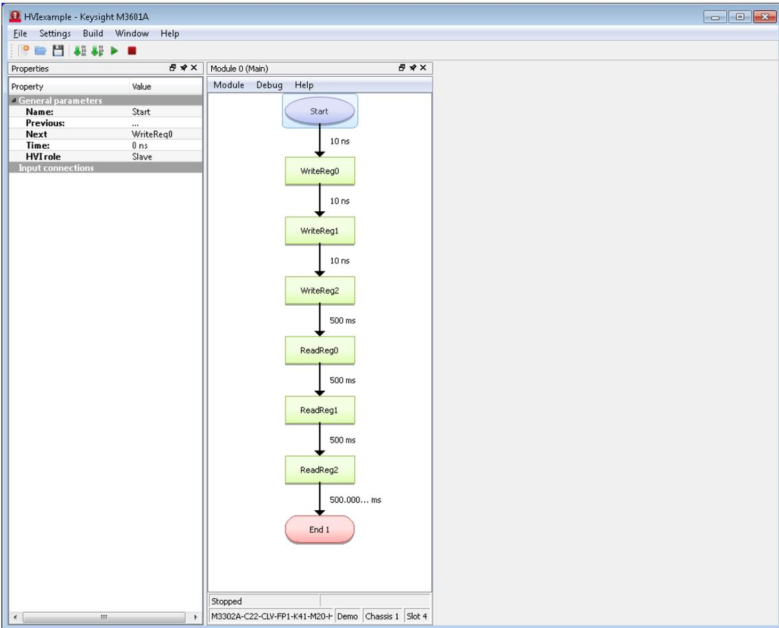
The HVI project comes setup to use the M3302A demo module. To use the real hardware module select Module→Assign Hardware... and select your hardware module.
