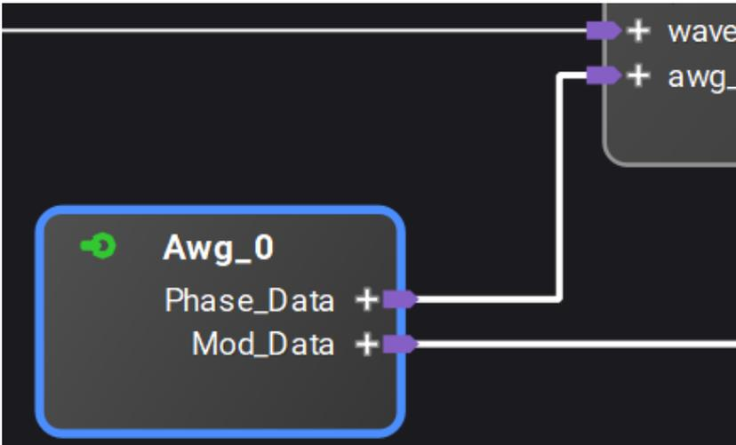
Clicking on the "+" sign for either interface will expand the interface to show the underlying ports. When an interface is expanded, clicking the "-" sign will collapse the port back to showing just the interface name.
