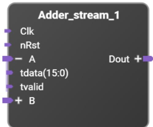
When the "A" interface is connected to the output of a compatible interface, all individual signals between the two interfaces are connected. If the design requires connecting an interface to an incompatible interface or individual ports on another block, the ports within the interface may be connected instead.
