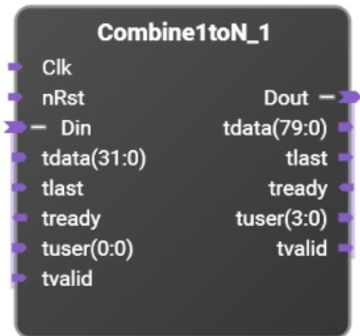
To convert a real, non-supersampled 16 bit data sample to a 5X supersampled 80 bit data stream is straight forward. For every five 16 bit input samples, one 80 bit output is generated. Things are more complicated when dealing with complex data. In that case, the input is 32 bits wide (16 bits of real data, and 16 bits of imaginary data). To convert this to 80 bits wide, 2-1/2 input samples are collected for each output. So for an input of:
