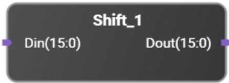
Signal shifter with configurable input size, direction and number of shifts.
