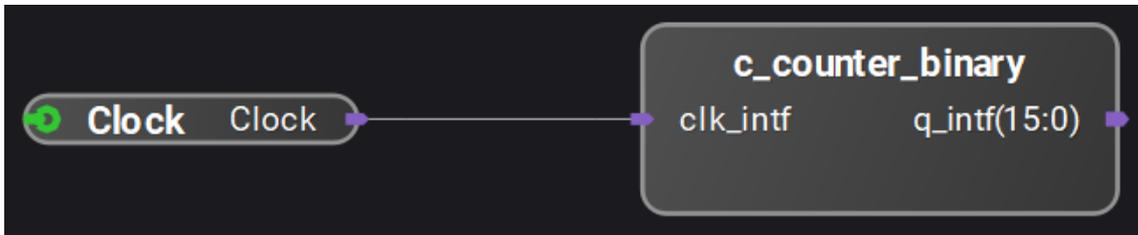
The counter was customized from the Vivado IP Catalog, imported into PathWave FPGA, instantiated in the design, and then connected to the Design Interface clock.
