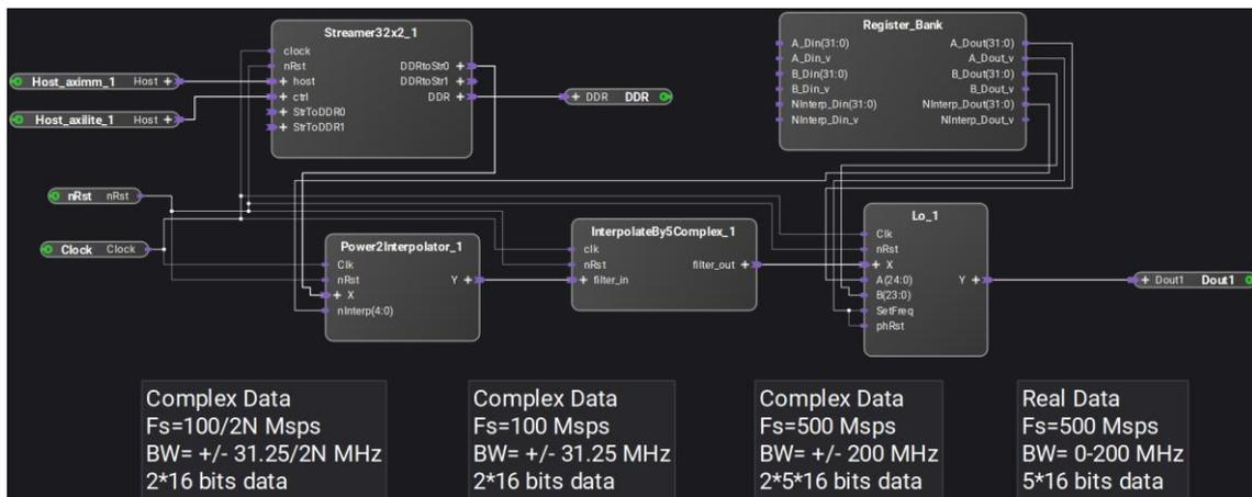
Following the signal flow from the output back towards the input, the output DACs of the M3302 are running at 500 Msp. The FPGA only runs at 100 MHz, so the output (Dout1) presents 5 DAC samples every FPGA clock. This is called supersampling by 5. The five 16-bit output samples are combined into one 80 bit wide AXI-streaming bus.
