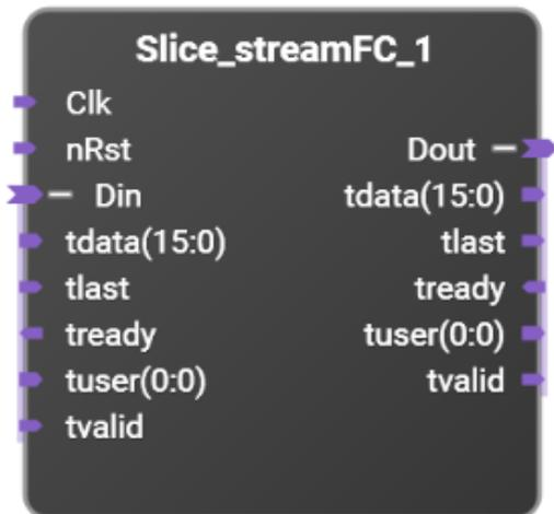
Streaming version of the slice block supporting full flow control.
