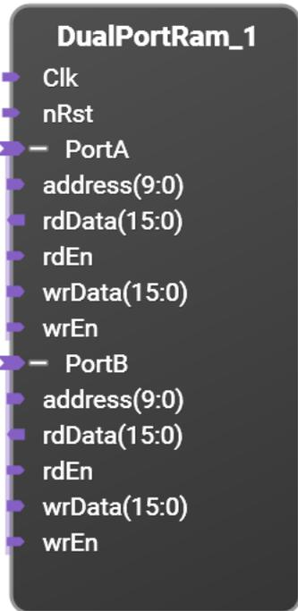
Dual port Block Ram up to 1024 bits x 65536 positions using PC MEM interfaces.
