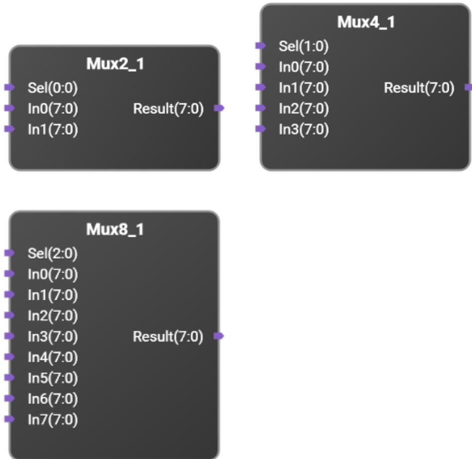
These are 2 to 1, 4 to 1, and 8 to 1 multiplexers. The value of the Sel input determines which of the various In ports connect to Result.
