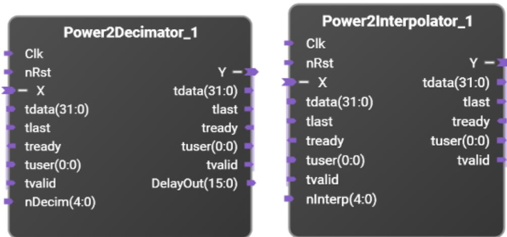
Conceptually, the Power2Decimator can be thought of as a set of 16 cascaded decimate by 2 stages (the internal design uses a more efficient architecture). Each stage first low pass filters its input and then decimates by two. A MUX controlled by nDecim selects the output of one of these filters.
