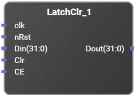
Latch with clock enable and synchronous clear.
