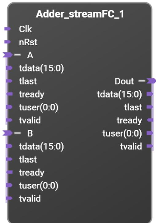
Signed adder with streaming interface with full flow control support.
