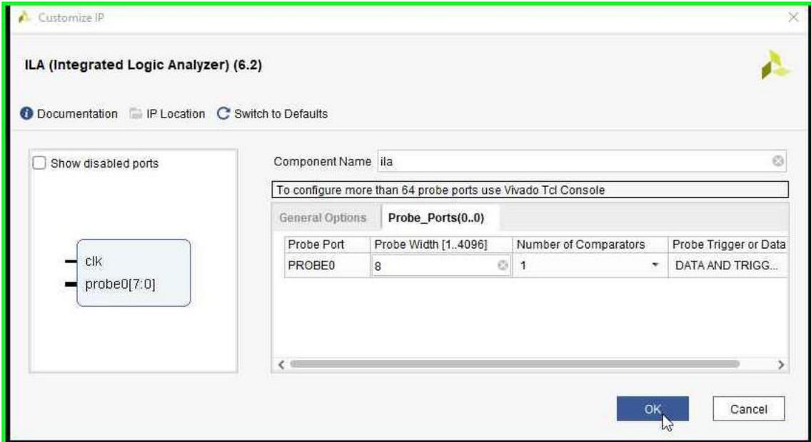
There is already 1 probe by default. Click on the Probe/Ports tab and set the probe width to 8 corresponding to the 8-bit counter in the design. Then, click OK. Next Vivado IP Manager will ask whether to generate the output products for the customized IP.
