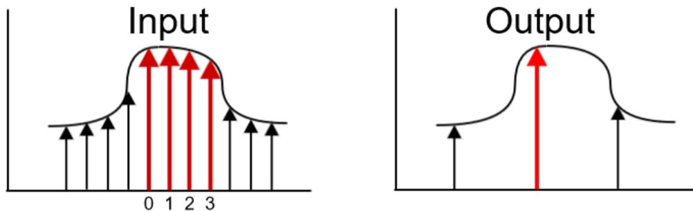
For example, if the filter is decimating by a factor of four there is only one output sample for every four input samples. A trigger for any of the four red input samples would result in the same red output sample being marked. The DelayOut value indicates which of these four actually caused the trigger event. A DelayOut value of 0 means the first red sample caused the trigger event. A value of 1 means the next red sample caused the trigger event, etc.
