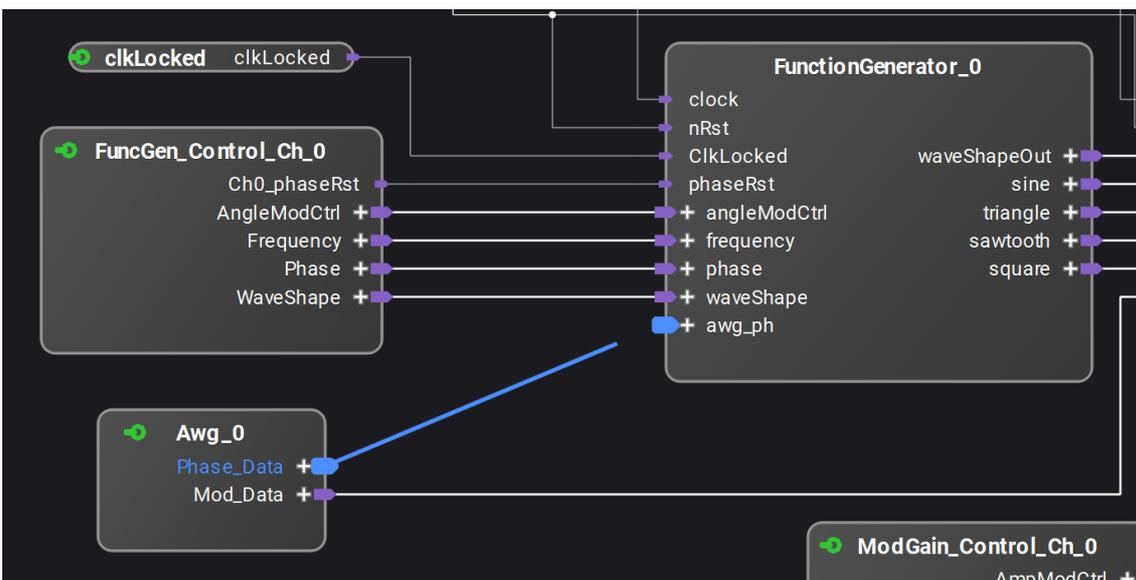
For finishing the connection, the end of the connection line is dragged by the mouse to a compatible target connector. In this case, the mouse icon changes to the green connection icon.
