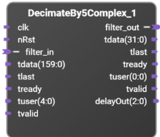
Decimate a complex, 5x, supersampled streaming input by a factor of 5. Decimation is achieved using a polyphase, FIR filter. The real and imaginary parts of each sample are interleaved with the real part occupying the less significant (lower bit number) word. The lower order 16 bits of the output are real output data and the upper 16 bits of the output are imaginary output data.
