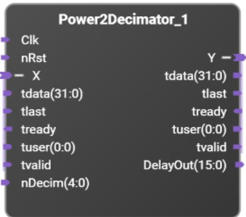
This is a power of two decimation filter that operates on complex data. It accepts complex data at up to one sample per clock. It filters and decimates the data by  $2^N$ , where  $N=0\dots16$ .
