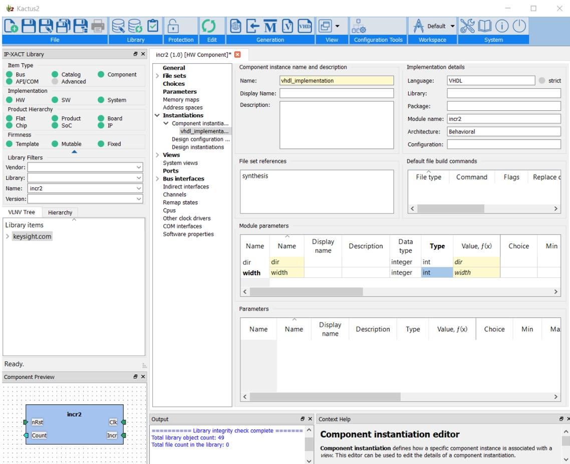
The definition of the IP block's interfaces and parameters is complete. If any of the entries in the middle pane are red (none are in this case), that would indicate that there is an error with that entry. Select it and fix any errors until none of the entries are red.
