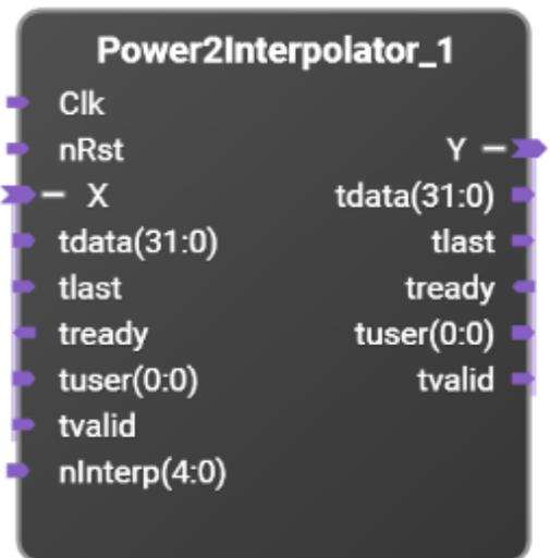
This is a power of two interpolation filter that operates on complex data. It accepts complex data and interpolates and filters the data by  $2^N$ , where  $N=0\dots16$ , generating up to one complex output sample per clock.
