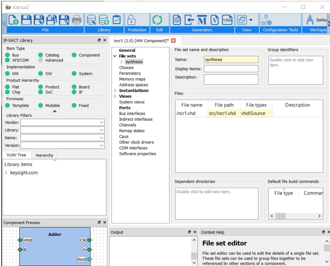
Now that the list of source files has been fixed, it is time to assign ports to logical *Bus Interfaces*. This allows PathWave FPGA to more easily connect interfaces between IP blocks. Click on **Ports** to bring up the Ports Editor. This should show all the ports that were read from the source HDL file and shows things like the direction (in or out), the width, and the index bounds for vectors:
