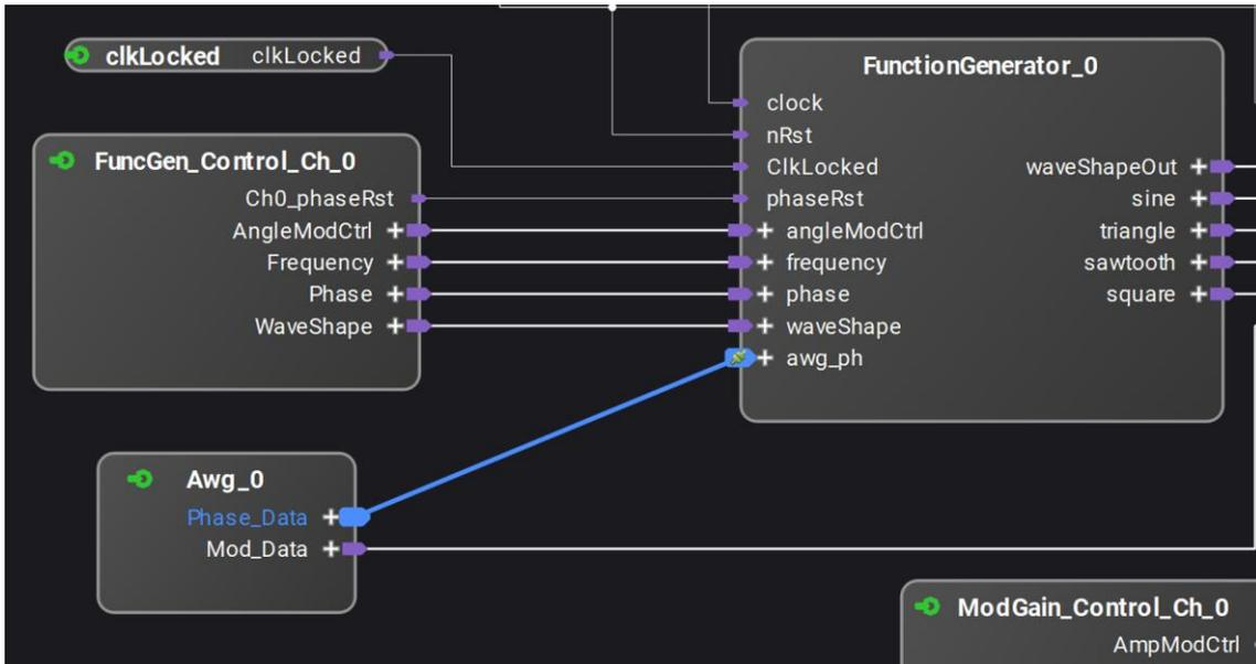
When the mouse button is released, the new connection is created.
