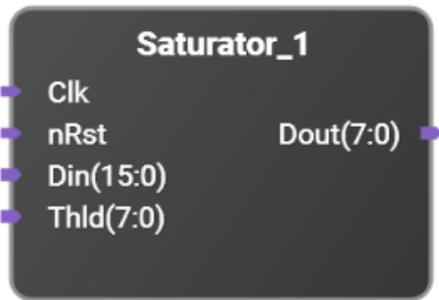
Output data is set to a saturation value (set by Thld port) whenever input data is equal or greater than that value.
