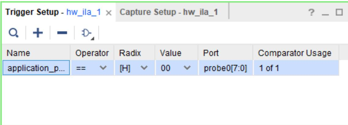
With the trigger setup above, the trigger position is stable on counter value equals zero condition.
