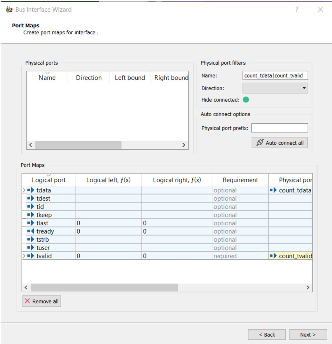
Click **Next** and **Finish** to complete the interface. At this point one can see that under the **Bus interfaces** section, all four of the IP block's interfaces are now listed.
