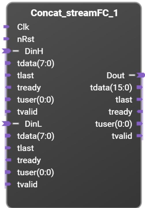
Streaming flow controlled version of the concat block.
