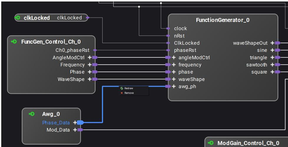
For example, add a block between the two ports. Notice the line connecting the ports is no longer straight.
