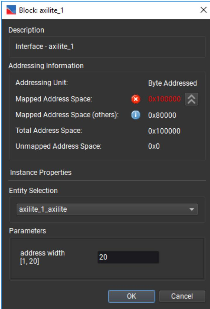
By adjusting the address width value of the new instance, the user can find the value that satisfies the space limits:
