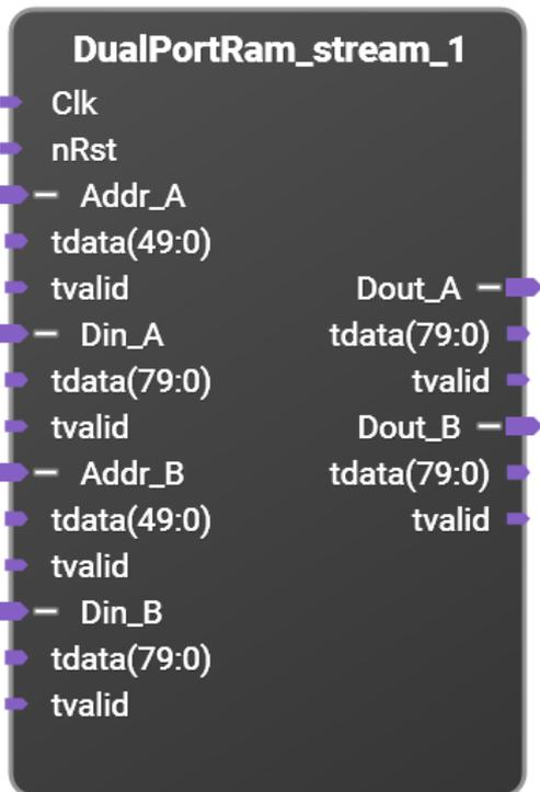
Dual port Block Ram up to 1024 bits x 65536 positions using AXI Streaming interfaces.
