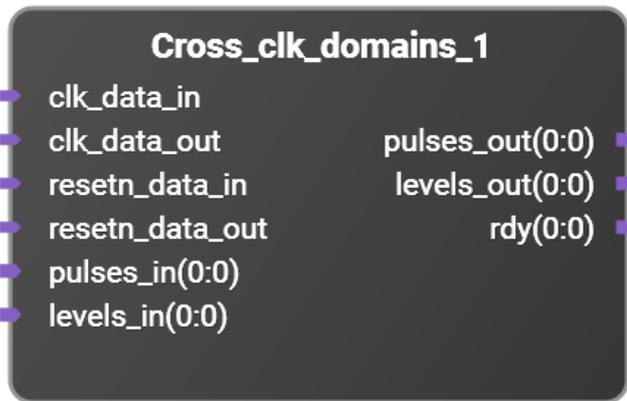
Logic to handle the crossing of signal levels and pulses to and from arbitrarily related clock domains.
