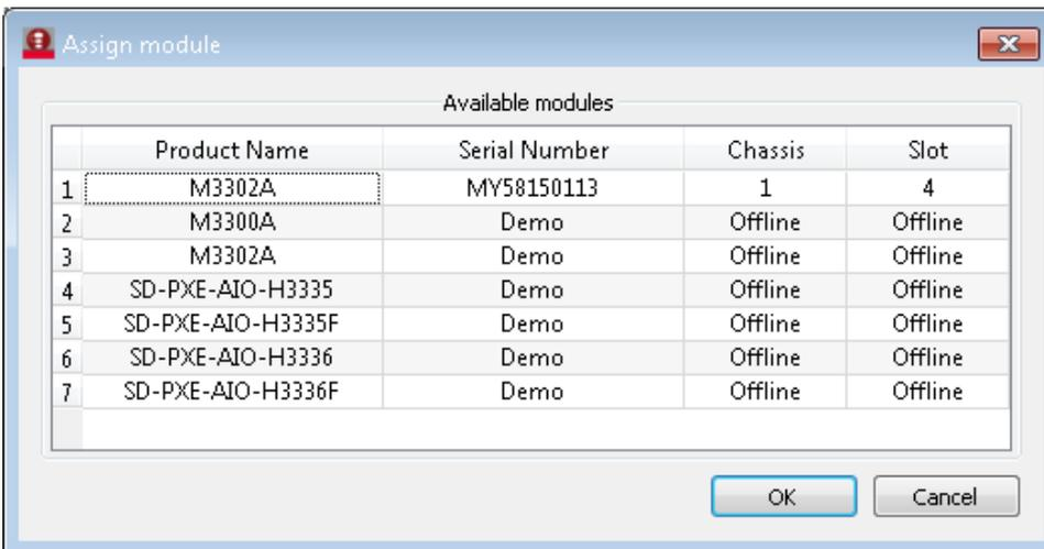
Load the FPGA bitfile onto the M3302A by selecting Module→FPGA→Load firmware...
