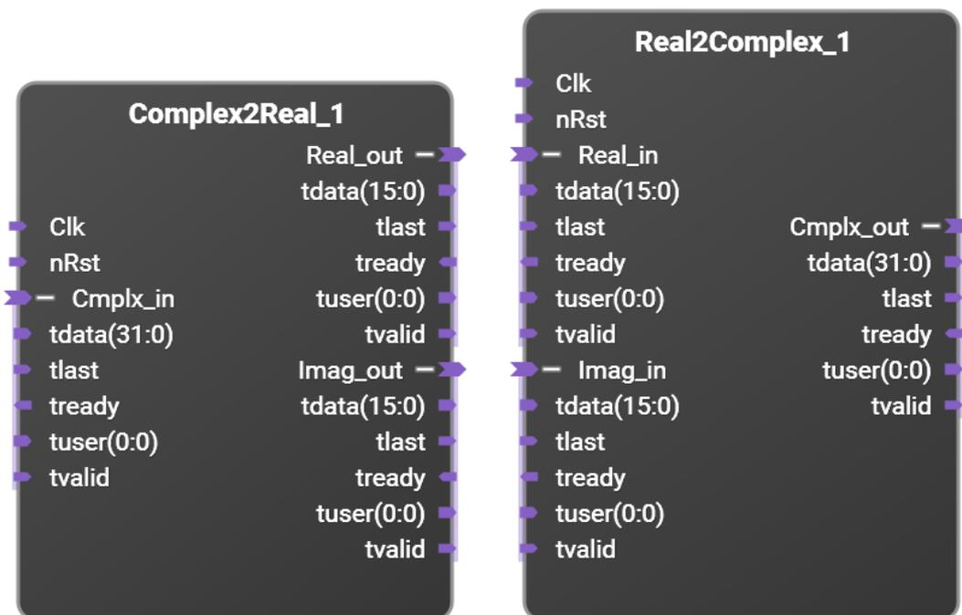
In order to know how to correctly interleave the complex data, these blocks need to know the size of the real data sample and any supersample value. The above pictures show a "Tdata size" of 16 and a "Supersample" of 1 (no supersampling). This means that the Real and Imaginary tdata busses are 16 bits wide, and the Cmplx tdata bus is twice this or 32 bits wide.
