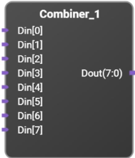
Combines N single-bit inputs into a single N-bit output vector.
