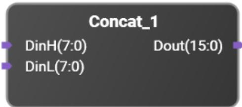
Concatenates two input signals into one single signal. DinH is the most significant half of Dout, and DinL is the least significant half of Dout.
