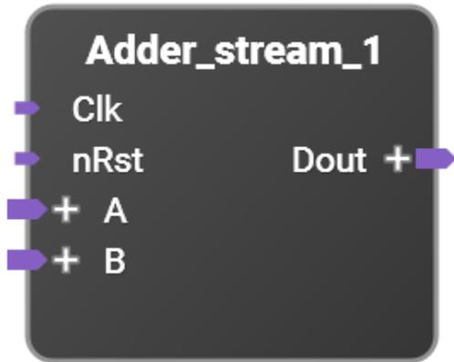
In the example above, this block has inputs to the left (input connectors point into the block), and outputs to the right side of the block (output connectors point out of the block).
