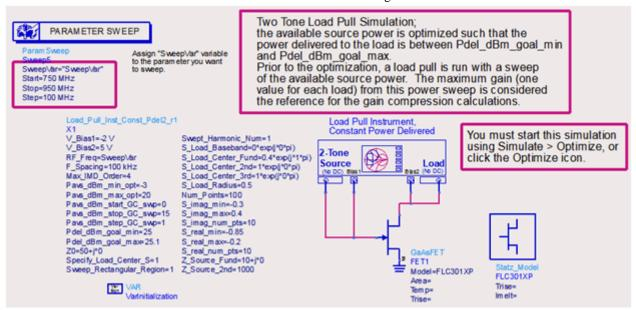
Here also you have to replace the sample device with yours and adjust the bias voltages as needed. You have to assign the swept variable SweepVar to some parameter on the schematic. In addition to all the other variables that you must specify as before, you need to specify the following two variables:
