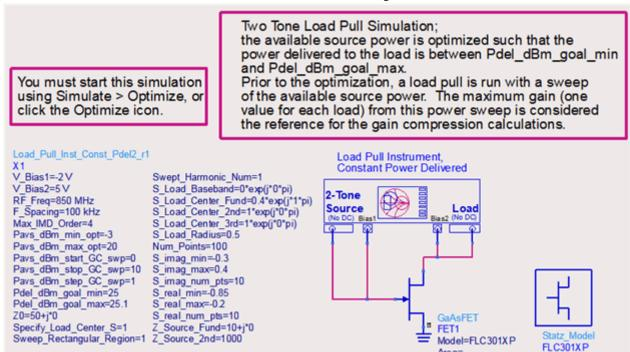
Here also you have to replace the sample device with yours and adjust the bias voltages as needed. In addition to all the other variables that you must specify as before, you need to specify the following two variables:
