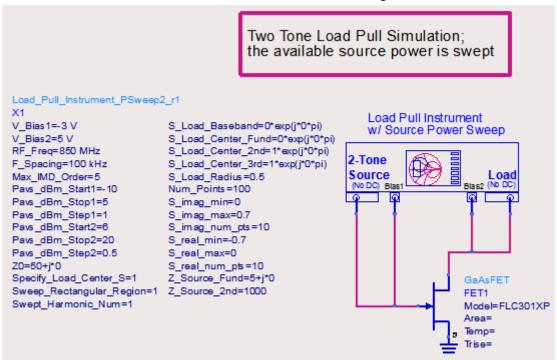
Here also you have to replace the sample device with yours and adjust the bias voltages as needed. In addition to all the other variables that you must specify as before, you need to specify the following two variables:
