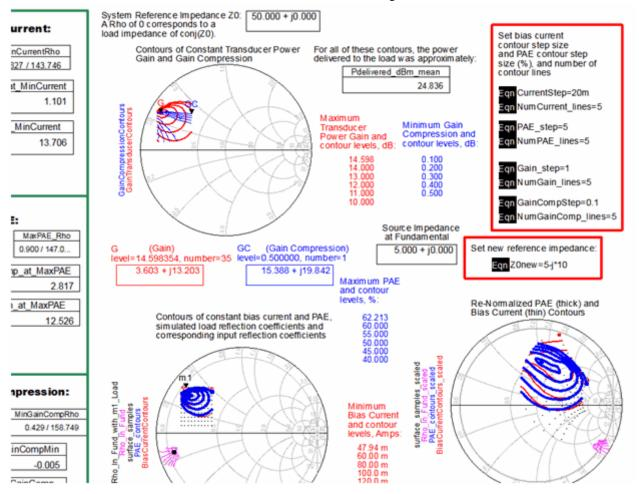
To see the contours effectively, you may need to change the CurrentStep, PAE\_step, Gain step, and GainCompStep variables. These set the step sizes between the contours.
