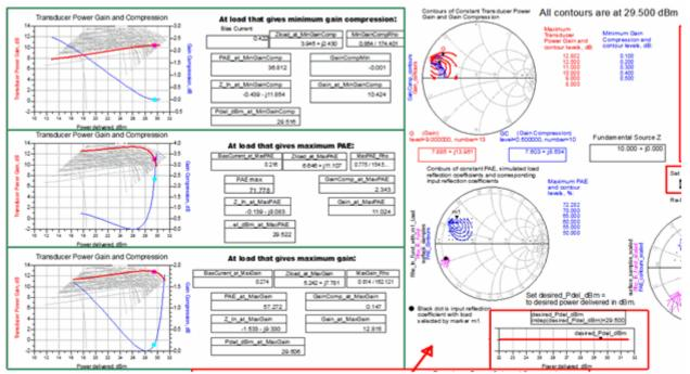
The data display shows the transducer power gain, gain compression, power delivered, and PAE contours for a particular power delivered to the load that you select using the desired\_Pout\_dBm marker. The gain and gain compression curves that correspond to several optimal load points (for minimum gain compression, maximum PAE, and
