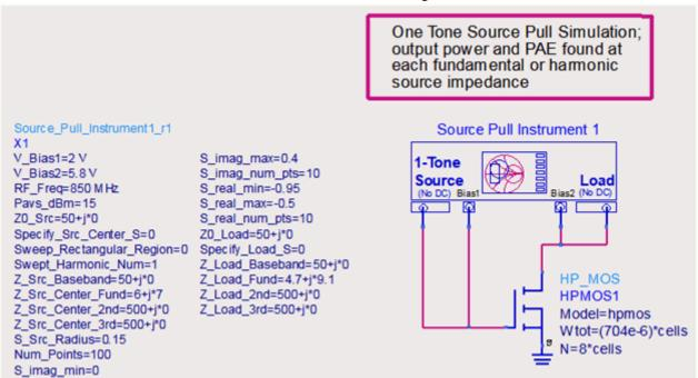
In this case, since the  $Sweep\_Rectangular\_Region=0$ , sweep a circular region of the Smith Chart. Also, since  $Specify\_Src\_Center\_S=0$ , we are using the  $Z\_Src\_Center\_*$  to specify the impedances at the fundamental and harmonic frequencies. Since  $Swept\_Harmonic\_Num=1$ , we are sweeping the reflection coefficient at the fundamental frequency.
