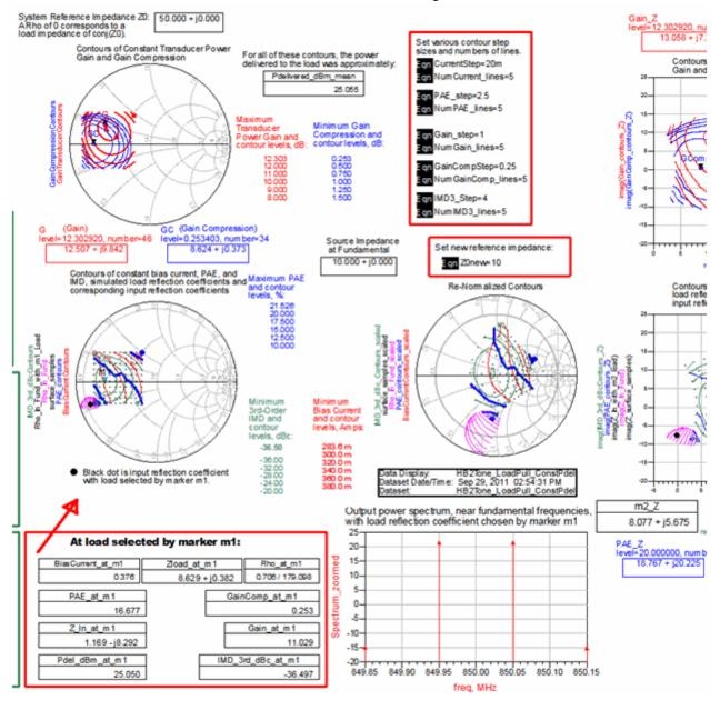
There is a clear trade-off between PAE and distortion. For this bias point, if you want maximum PAE, you suffer a lot of gain compression and intermodulation distortion.
