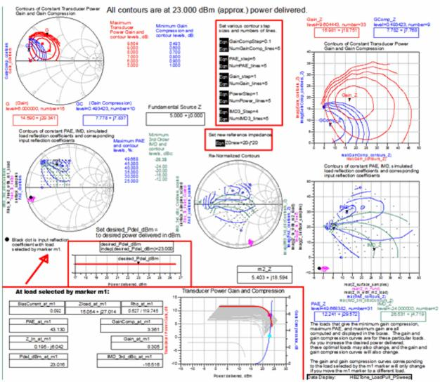
From the same swept-power simulation results, you may see gain compression contours by selecting **DesignGuide > Load Pull > Display Contours at X-dB Gain Compression**. Note that there are two such menu picks. The lower one is for displaying results from a two-tone simulation, whereas the upper one is for a one-tone simulation.
