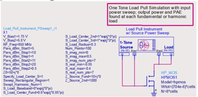
In addition to the various settings done in the **HB1Tone\_LoadPull** schematic, you also have to specify the sweep limits for the *Pavs\_dBm* variable. Here we have two ranges, one with a coarser step (assumed to be the linear region) and one with a finer step (in the compressed region.)
