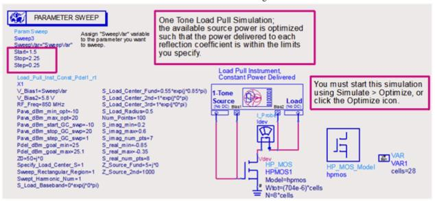
You have to assign the swept variable *SweepVar* to some parameter on the schematic as well as set its sweep limits. In this case, the gate bias voltage V\_Bias1 will be swept from 1.5 to 2.25 Volts. After running the optimization, open the
