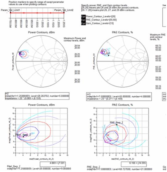
The above plots show how the region of load impedances required to obtain 28 dBm power delivered gets much smaller as the input frequency increases. When plotting contour lines as a function of a swept parameter, they may be easier to interpret if just one or two contour levels are specified.
