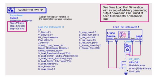
The above figure specifies the limits of the swept variable, *SweepVar*, and assigning it to RF\_Freq. The corresponding data display has plots similar to the ones shown earlier, but it also has a page with contours at multiple values of the swept parameter.
