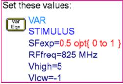
During the optimization, this variable is adjusted within the limits until the power that you want is delivered to the load.
