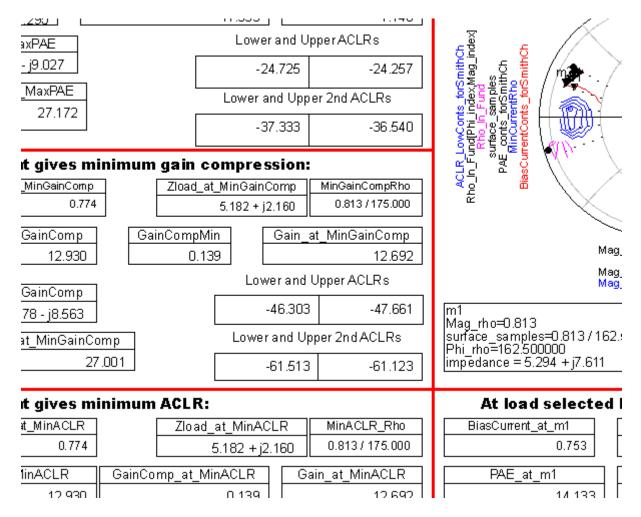
To see the contours effectively, you may need to change the *CurrentStep*, *PAE\_step*, *Gain\_step*, *Gain\_compStep*, and *ACLR\_step* variables. These set the step sizes between the contours. The bias supply current calculations only include the current in the probe *Is\_high*. If you change the name of the current probe, you will need to edit the BiasCurrent equation on the Equations page.
