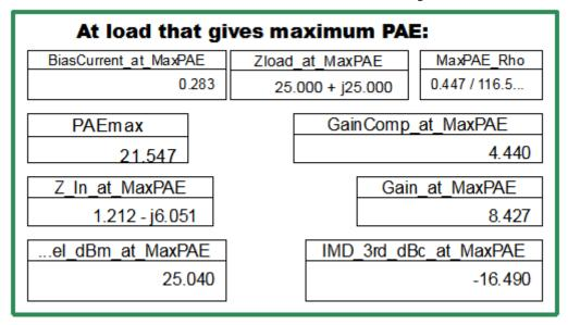
Tolerating a lower PAE allows much lower gain compression and intermodulation distortion.
