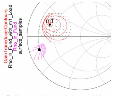
Black dot is input reflection coefficient with load selected by marker m1.
