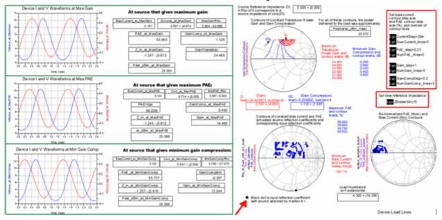
To see the contours effectively, you may need to change the PAE\_step, Gain\_step, and GainCompStep variables. These set the step sizes between the contours.
