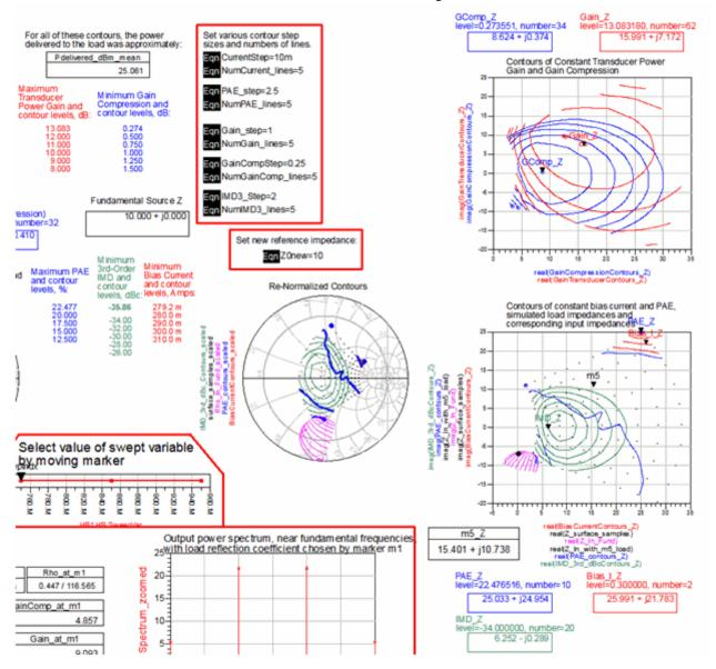
There is a clear trade-off between PAE and distortion. For this bias point, if you want maximum PAE, you suffer a lot of gain compression and intermodulation distortion.
