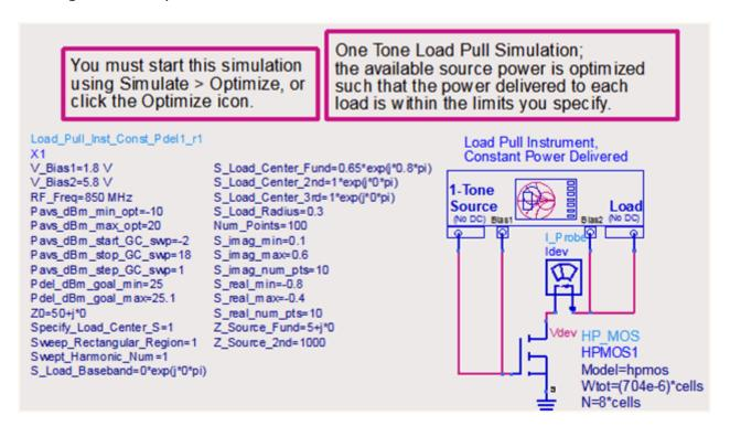
You have to make the same types of edits to this schematic as with the others described above. Also, you have to specify the minimum and maximum allowed values of the available source power, Pavs dBm min opt and Pavs dBm max opt, respectively.
