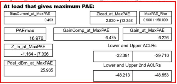
Note that the power delivered specification is not satisfied. You could re-run the simulation, allowing SFexp to vary over a larger range, or you could move marker m1 to a load near this one and see if the power delivered specification is satisfied. Moving marker m1 allows you to select any of the simulated load reflection coefficients. The corresponding data appears in a separate box, which allows you to see potential tradeoffs as you move around the Smith Chart.
