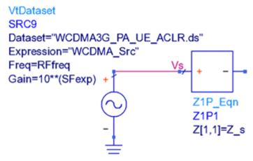
It is not obvious what the relationship is between this exponent and the available source power. However, the  $WCDMA\_SrcTest$  schematic in the same workspace allows you to sweep this scale factor and calculate the corresponding available source power. In this case, stepping SFexp from -1 to 1 increases the available source power from about -20 dBm to +20 dBm. This does vary with the source impedance you specify.
