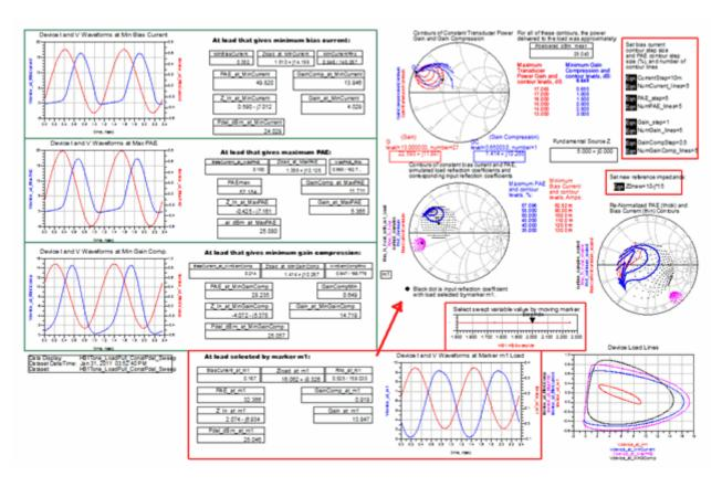
All the data is now indexed to the swept parameter value, which you select by moving the SweepIndx marker. There is a change in the power-added efficiency as you change the bias voltage.
