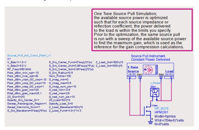
Relative to the other constant power delivered simulation schematics above, the only difference is that you have to specify the constant load impedance at the fundamental frequency, instead of the source impedance. You may also specify different load and source impedances at the harmonic frequencies. Typically, you would first run a load pull simulation to determine the fundamental load impedance to use here.
