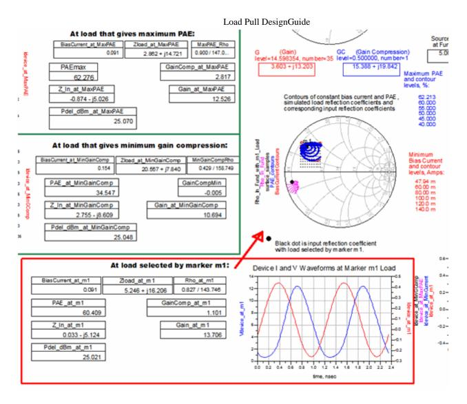
Data within the red box corresponds to the reflection coefficient selected by marker M1.
