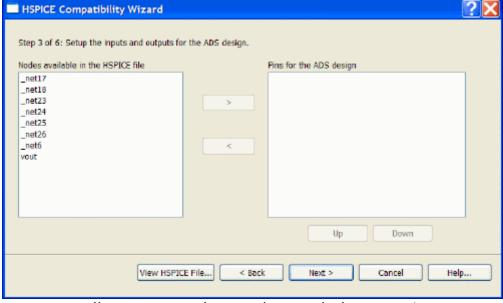
6. The next page allows you to choose the symbol generation parameters. Based on the terminal setup page (or on the .subckt terminal definition for the circuit that was chosen), the pins for the ADS design is populated. This is a non-editable field. To change the order or pins you must go back to the appropriate prior page using the back button.
