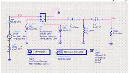
All simulation directives in the HSPICE file are ignored. You must place ADS simulation components in your design to perform simulations.
