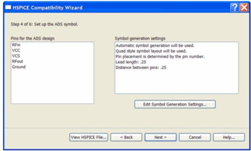
To change the settings, click **Edit Symbol Generation Settings**. This displays the standard ADS auto-generation dialog for symbols. When finished, click **OK** to update the summary. These settings will be used to generate the symbol when the wizard is finished.
