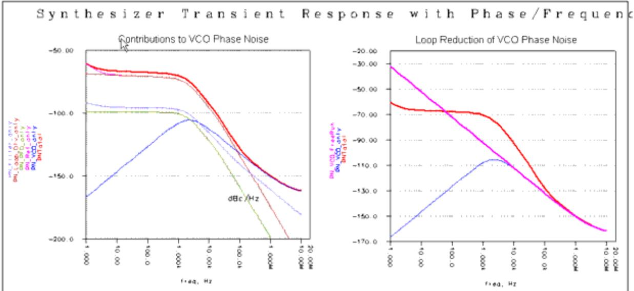
The graph on the left displays the individual noise source's contributions and the graph on the right shows the overall noise performance of the PLL.
