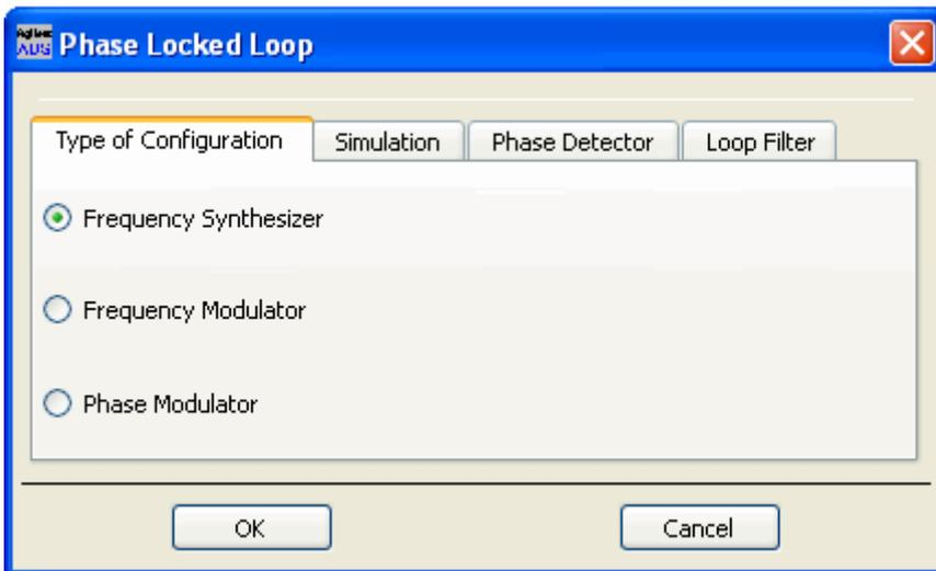
You can select one of the available PLL configurations as shown below. Having identified the type of PLL structure, you then select one of the three simulations available from the **Simulation** tab, as shown here. The simulations include *Loop frequency Response*, *Phase Noise Response*, and *Transient response*.
