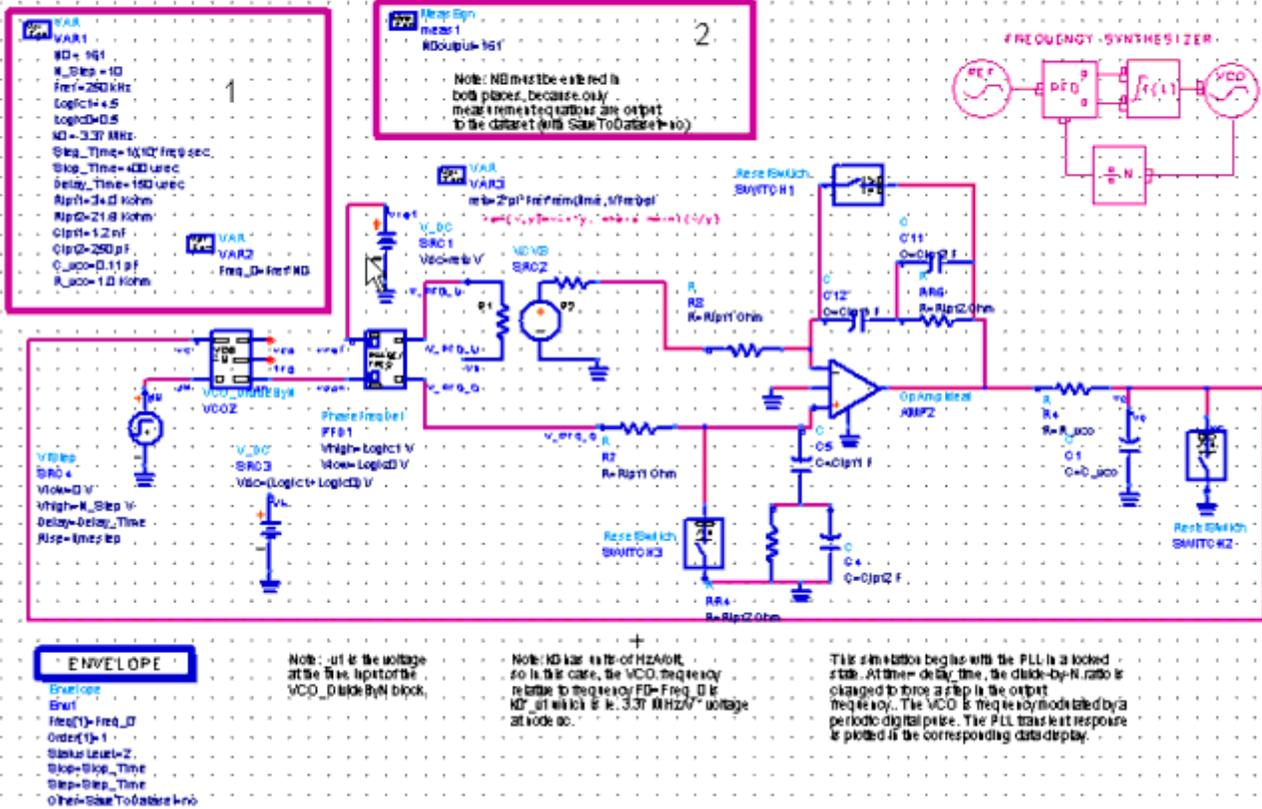
The loop filter parameters derived from the Loop Frequency response need to be entered into this schematic, along with the VCO and Phase Detector constants. The transient response requires additional parameters such as the Reference Frequency and the stop and delay time, as well as the Divider Ratio step change.
