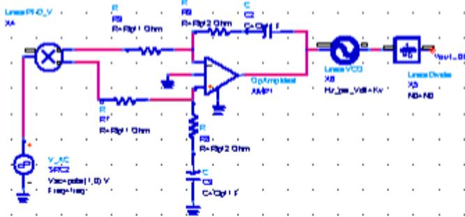
Loop Filter Frequency Response Simulation
