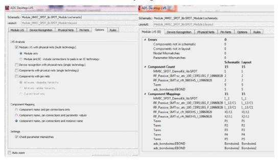
Module LVS at IC level checks if the bond pads are shorted in the MMIC layout (using mapped layers).
