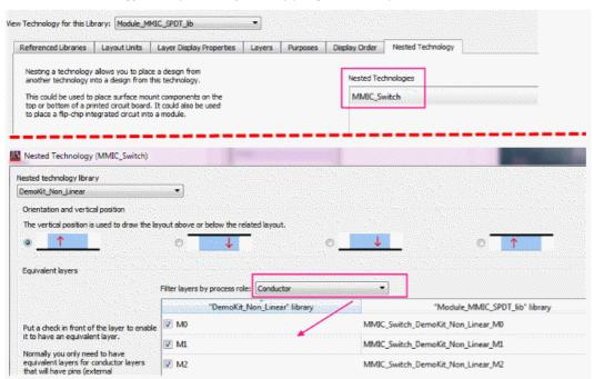
All the metal layers of MMIC substrate are mapped to the Module substrate. View of Module Substrate
