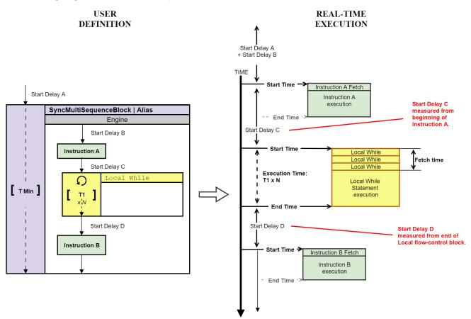
The following diagram shows a while loop that generates an error:
