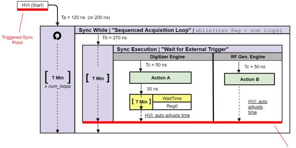
Triggered-Sync Point The following diagram shows the execution timeline for the first 3 iterations of the sequence shown in the previous diagram:
