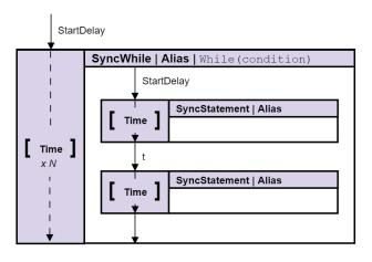
If you are using a Sync while statement across multiple engines, during its execution, one of the engines is set to the role of *Primary* and the remaining engines have the role of *Secondary*.
