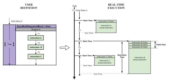
The following diagram shows an example with two local instruction statements and the timing when executed by the HVI engine.
