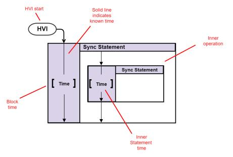
Local Sequences are placed within their Engines in Sync multi-sequence blocks. The following diagram shows a pair of Local Sequences with an instruction each inside a Sync multi-sequence block:
