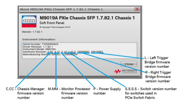
The following screenshot shows a breakdown of components of different versions of the M9019A chassis firmware:
