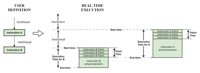
NOTE It is important to consider the effects of overlapping instructions execution, because the result of the first instruction is not effective or available when the overlapping instruction finishes its fetch cycles and starts execution.
