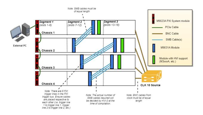
NOTE Ensure the SMB cables used to connect the M9031A modules are as short as possible. The chassis should be stacked in the same rack, on top of each other, and as close as possible to each other to enable the SMB cables that connect them to be as short as possible
